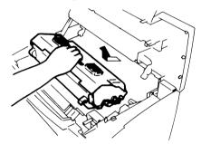
Take a new Imaging Cartridge out of the box. Holding it with both hands, shake it well in the directions indicated by the arrows.
